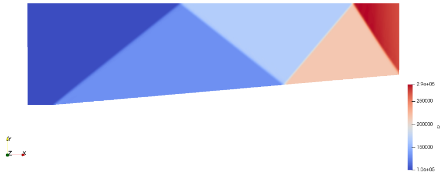
Figure 3. Steady-state flow pressure field for the rhoCentralFoam solver, \beta = 5^\circ
