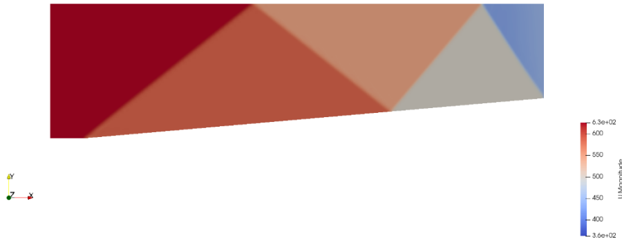
Figure 5. Steady-state flow velocity magnitude field for the rhoCentralFoam solver, \beta = 5^\circ
